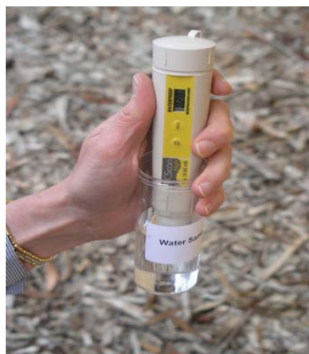
Figure 1. Testing water salinity using a salinity meter (Photo Elizabeth Madden).
