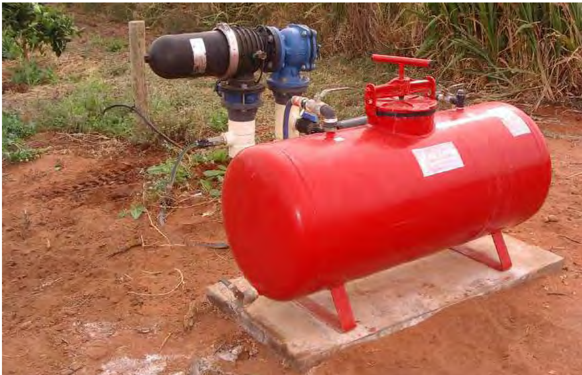
Figure 3. An in-field pressure differential tank.
