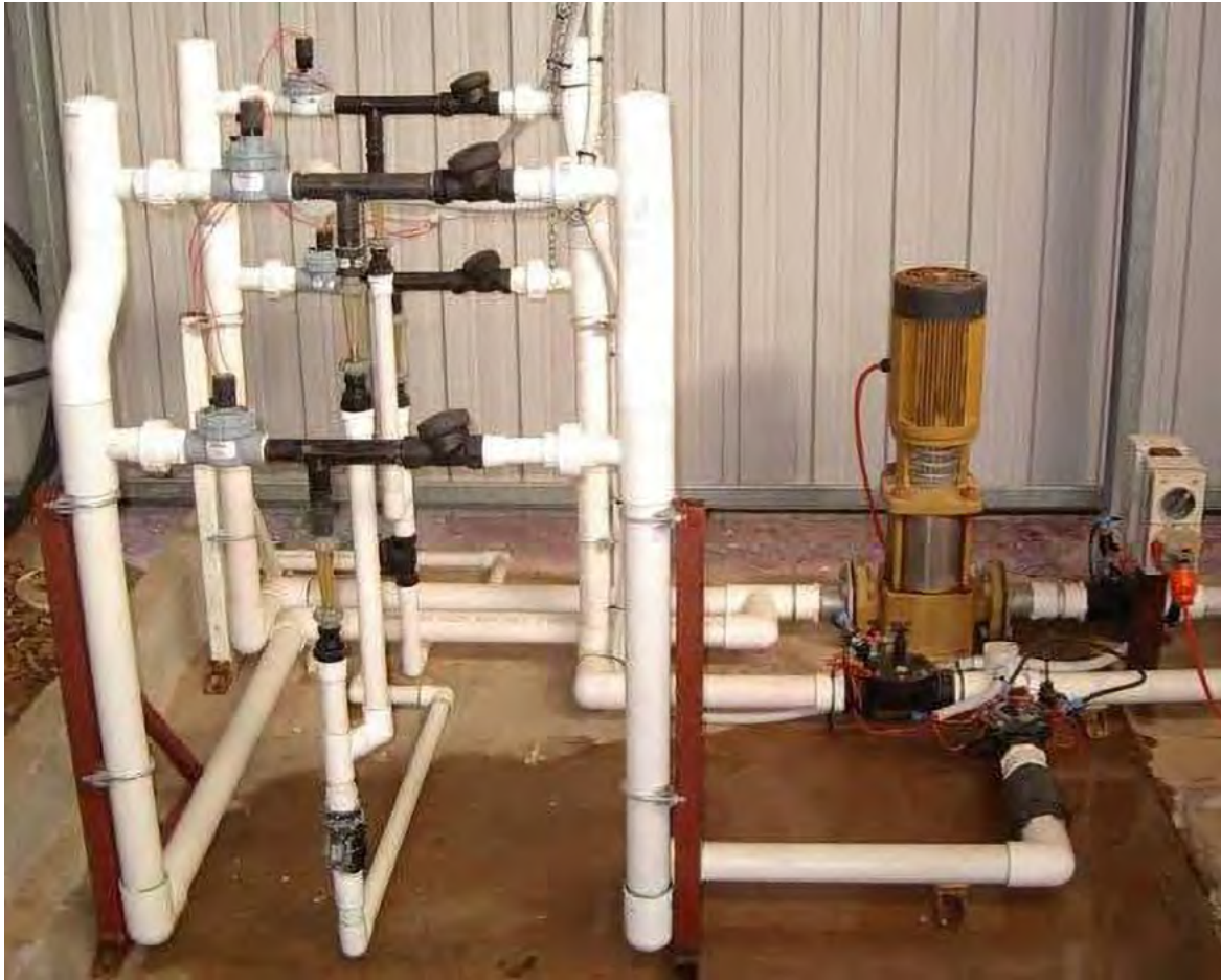
Figure 4. A do-it-yourself Venturi injection system operated by solenoid valves and an irrigation controller.
