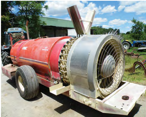
Figure 128. Deflectors on an air-blast sprayer. Photo: Deveau (2015).
