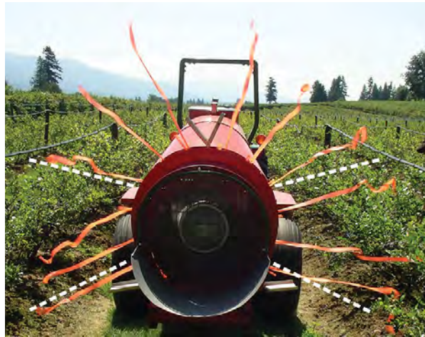
Figure 129. Using ribbons to work out where the air is being directed from the sprayer. Photo: Deveau (2015).
