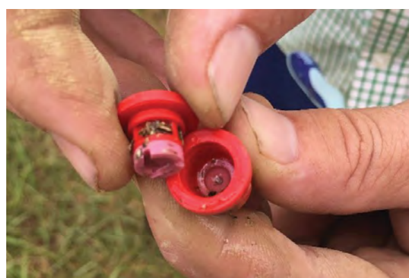
Figure 126. Regularly cleaning nozzles will improve delivery rates by removing debris build-up.
