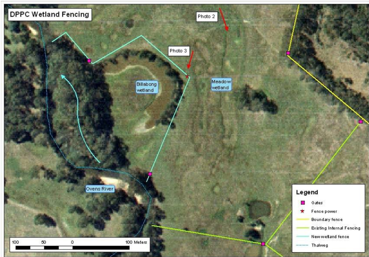
Map 2: The fence around this billabong wetland has been kept on the high ground, is as straight as possible, avoids overhanging branches and has been kept out of the flood channel (blue arrow). Gates are positioned so that cattle can be moved in and out easily for grazing when required. The numbered photo points (red arrows) refer to the photographs contained in this case study.
