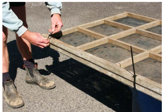
Figure 4. Spat bearing tray and lid tray being tied together through aligned holes drilled in the tray frames.
