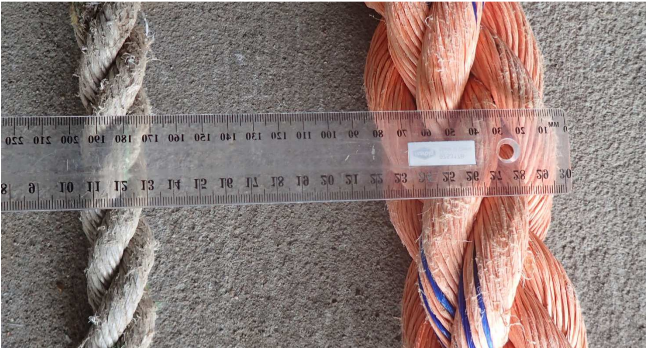
A 24mm rope next to the 44mm anchor deployment line used on the Research Lease (Source: NSW DPI, 2016) Note: Rope dimensions are measured with a load applied and these ropes are unloaded
