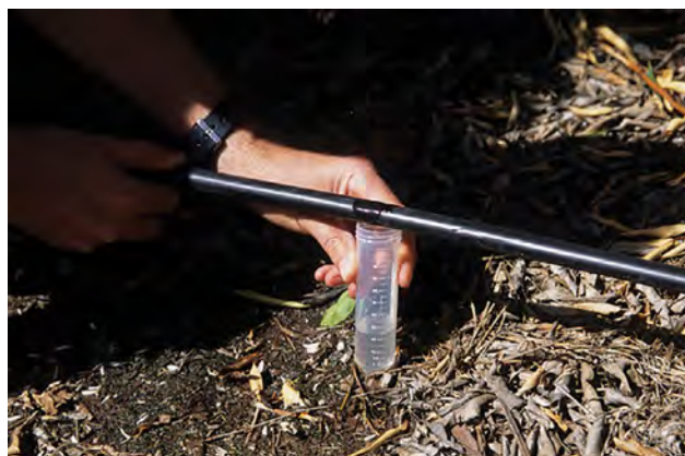
Figure 5. Measuring dripper discharge.
