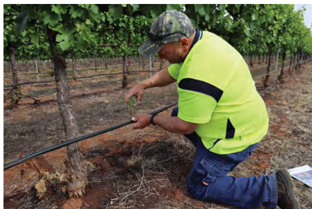
Figure 6. Measuring operating pressure.
