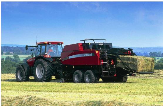
Figure 2: Adaptive driving may not necessarily be a factor for harvesters or tractors operating in predominantly power take-off mode, since the dominant power use is not related to driving style
