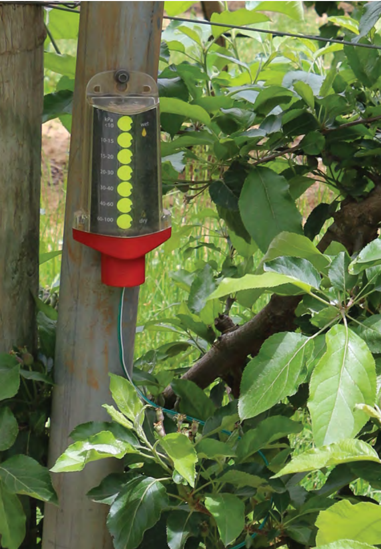
Figure 15. An example of a gypsum block probe.
