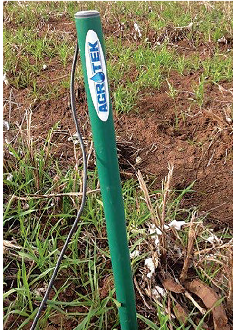
Figure 16. An example of a capacitance probe.
