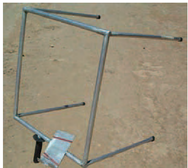
Figure 1. A 0.125 m 3 square counting frame with a notepad holder.
