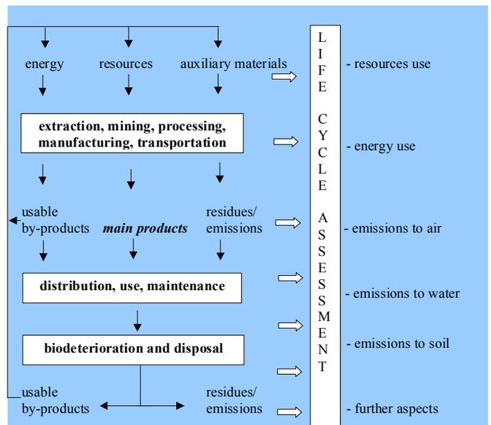
Figure 1. Diagrammatic representation of a generic LCA process
