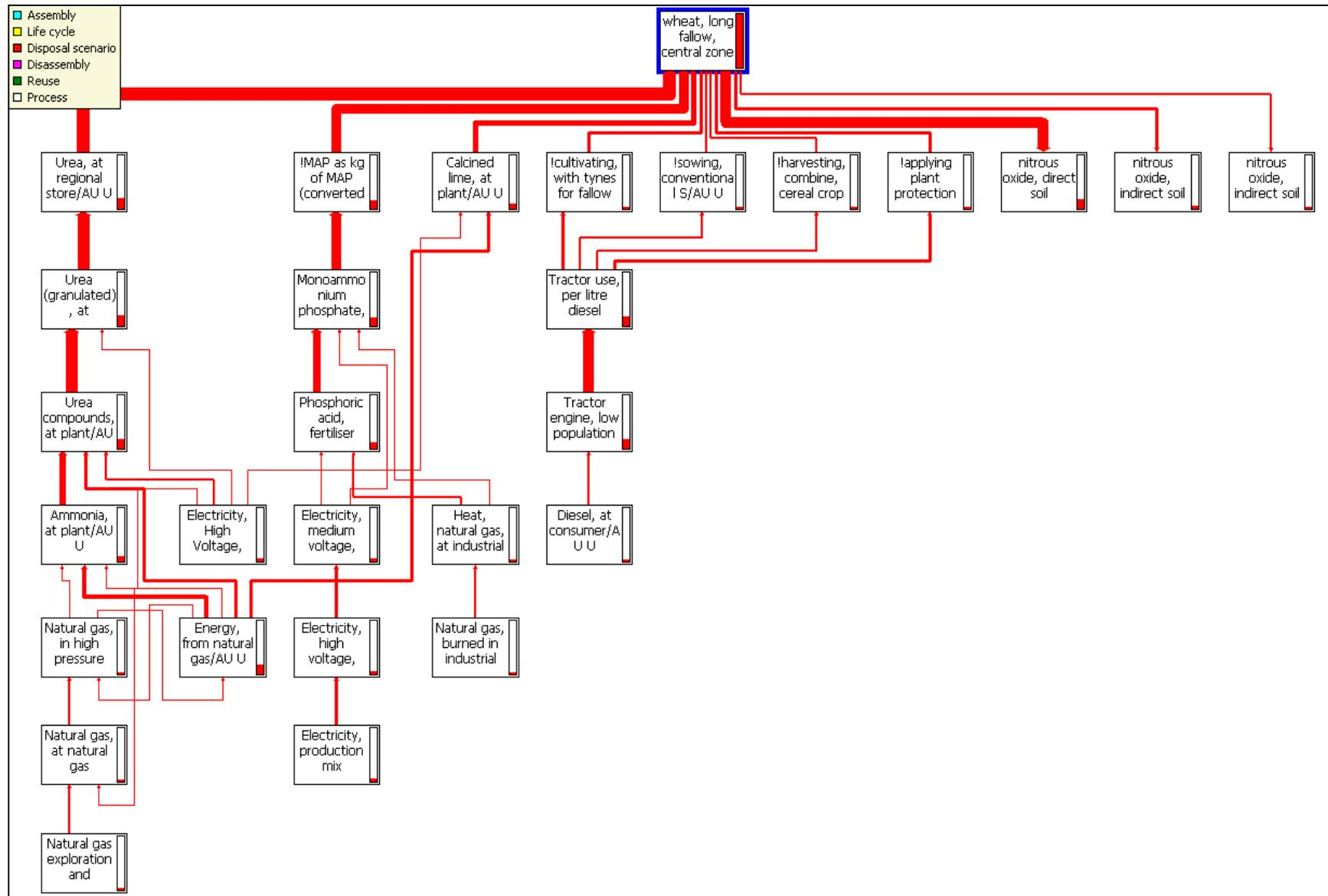
\* Not all emissions are visible, nor are all of the 2273 processes that comprise this LCA, as the cut-off has been set at 3.1% to simplify the diagram. The width of the branches represents the contribution from each process to the total emissions.
