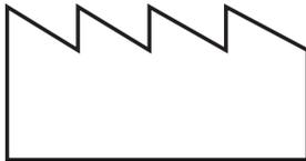
The sawtooth is erected with the vertical side of the ridges facing away from the prevailing wind. The design provides effective, natural removal of hot air from the greenhouse.
