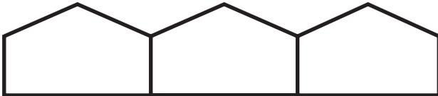
Multi-spans are efficient in terms of heat energy requirements because the total surface area is less than that needed for single spans of the same floor area. The distance from the sides to the centre of a multi-span, however, can present a ventilation problem and overheating can occur in the centre of a multi-span.
