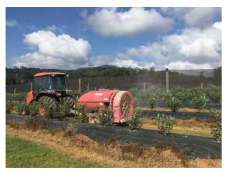
Figure 3. An axial air-blast sprayer. Photo: Melinda Simpson.
