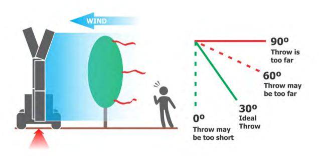
Figure 9. Using ribbons to determine adequate air speed for spraying. Source: Airblast 101 Handbook.
