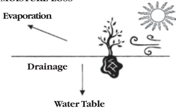
The two main sources of moisture loss are drainage and evaporation.
