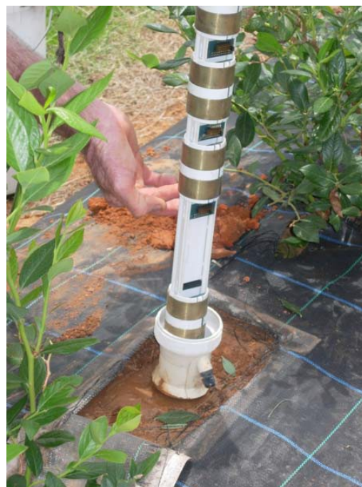
Figure 3 EnviroSCAN showing electronic sensors at various depths
