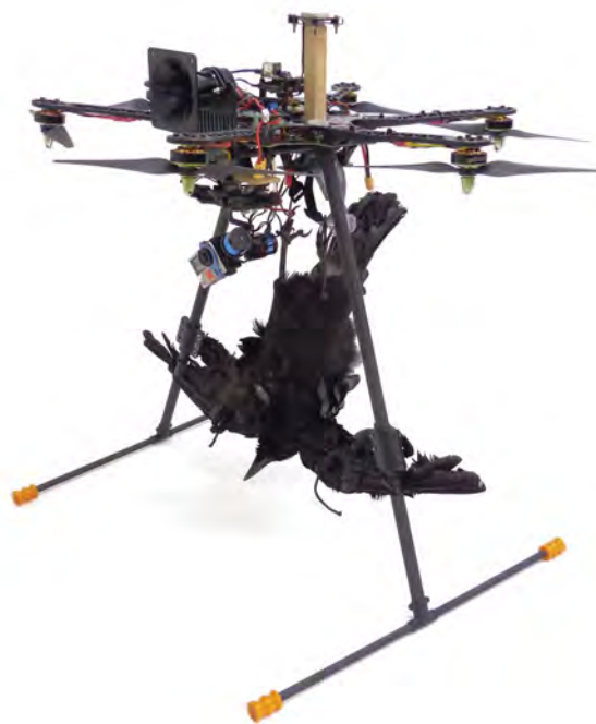
Figure 53. The unmanned aerial vehicle equipped with a horn tweeter (top left) and a crow taxidermy (bottom).
