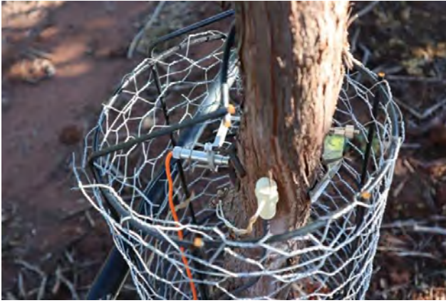
Figure 7. Dendrometer (side) and sap flow meter (middle) on a grapevine at the Griffith Research Station.
