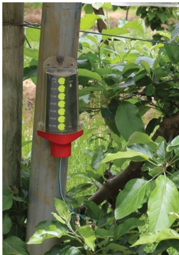
Figure 2. An example of a gypsum block probe.
