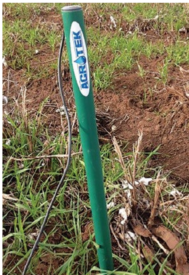
Figure 3. An example of a capacitance probe.
