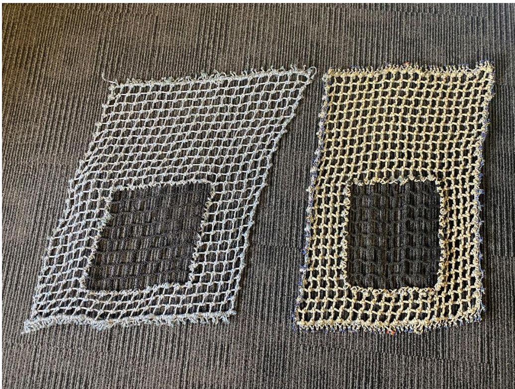
Figure 2: New Ocean square-mesh panel BRD (left) and another ~6 months old affected by extraordinary shrinkage (right).
