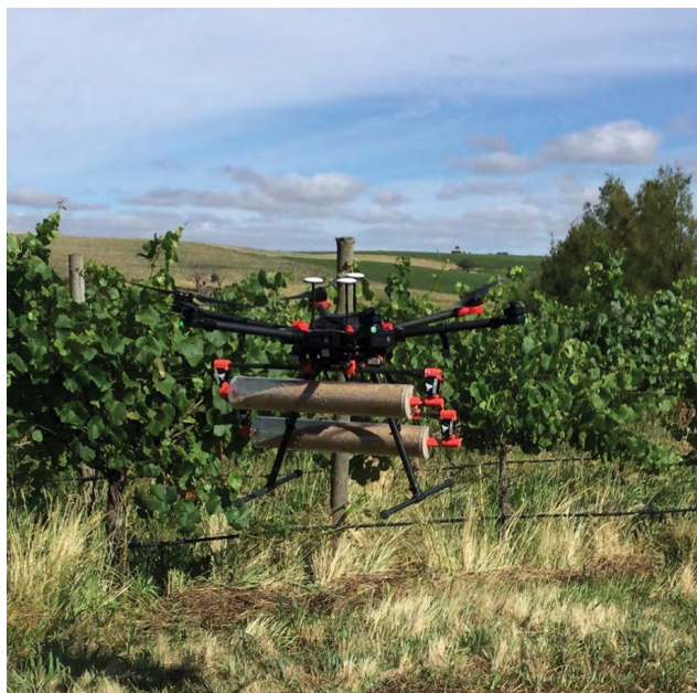
Figure 31. A drone releasing beneficial predatory mites over Nashdale Lane Wines, Orange. Photo: Darren Fahey, NSW DPI.
