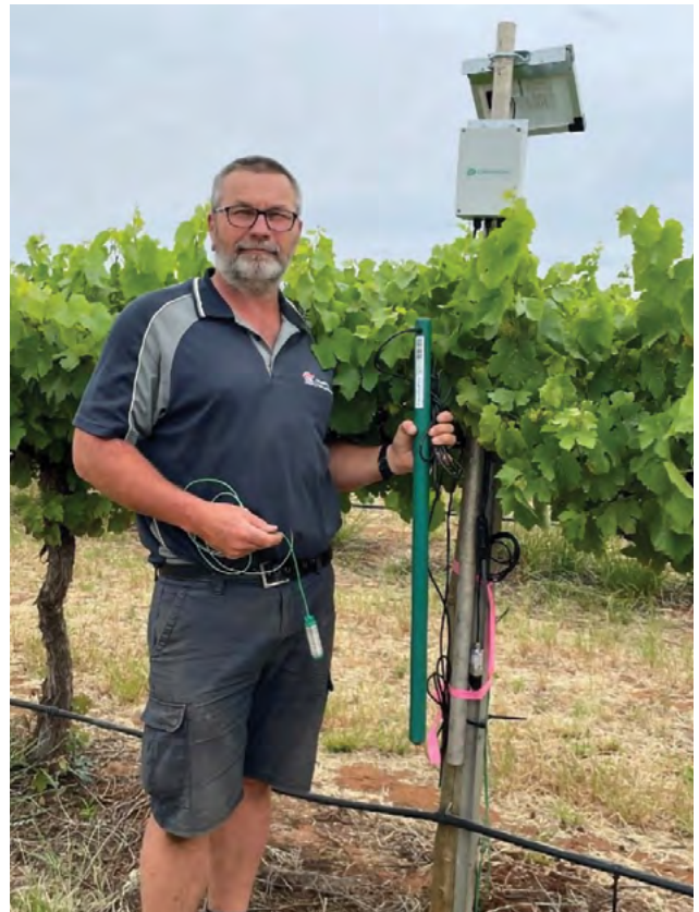
Figure 26. The Green Brain system installed in one of the Chardonnay blocks on the NSW DPI Griffith Research Station. Robert Hoogers is holding one of many Enviro Probes that were installed.
