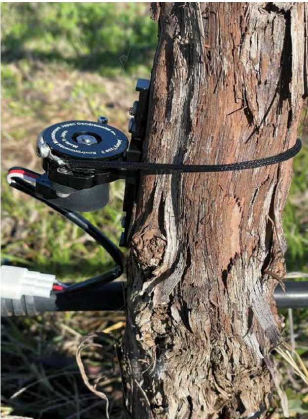
Figure 27. One of the many dendrometers to be installed in the viticulture and citrus blocks at the NSW DPI Griffith Research Station.
