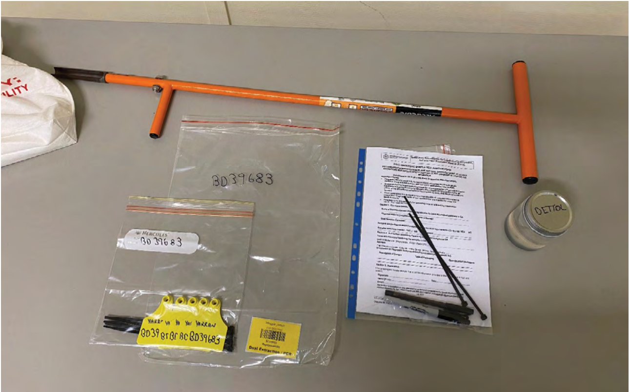
Figure 49. Sampling kit used for DNA probe method.
