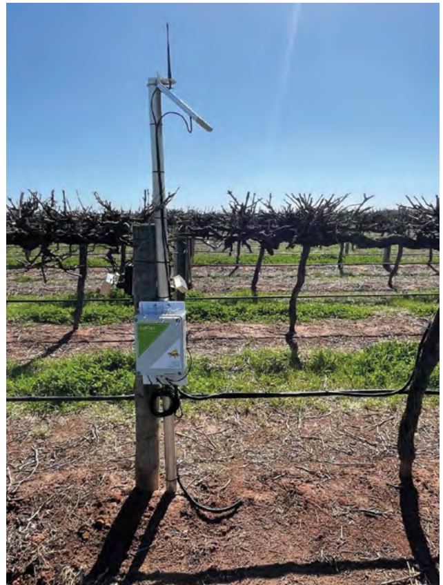
Figure 28. The receiver for the SupPlant system installed on the NSW DPI Griffith Research Station in a Shiraz block.
