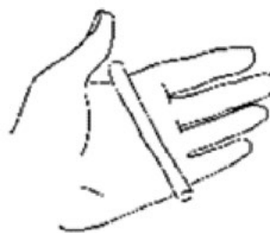
Figure 12. If a rod can easily be formed from a small soil sample, it is at risk of compaction.
