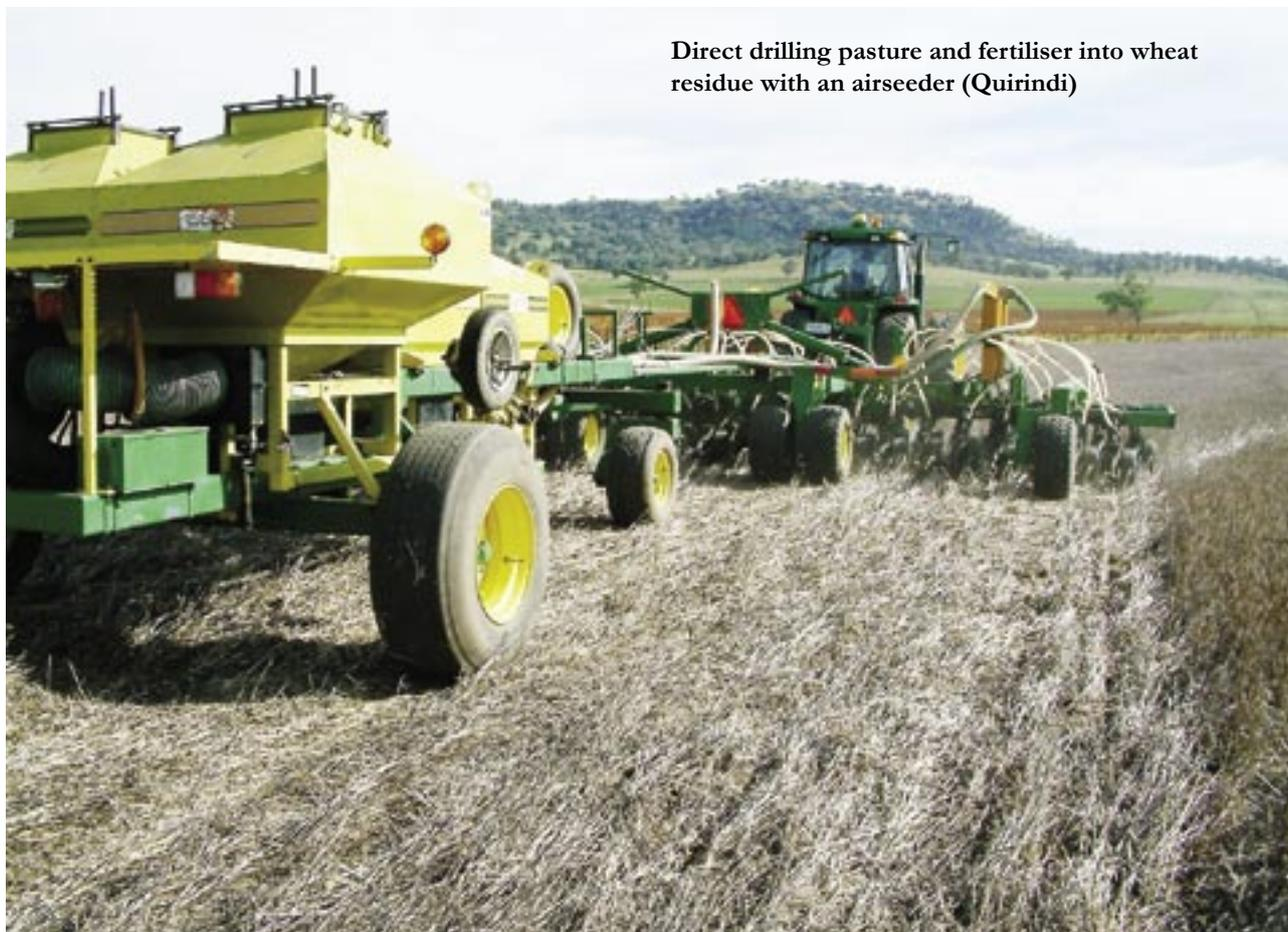
Direct drilling pasture and fertiliser into wheat residue with an airseeder (Quirindi)
