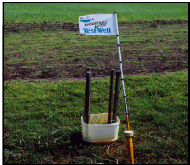
Fig 3. Test well used to monitor ground water level. (Picture by Christina Collins, 2002)
