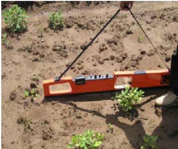
Fig 2. Poor establishment of crop on saline land in Pante Raja, Pidie. The EM38 instrument shown is used to assess the salinity level of this soil.
