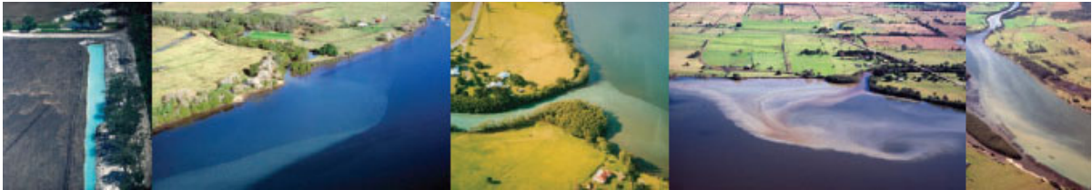
Figure 2. Acid sulfate soil outflows can also appear blue-green at pHs below 5, or milky white at pHs just above 5. This appearance is caused by the presence of very fine particles of aluminium minerals suspended in the water column.
