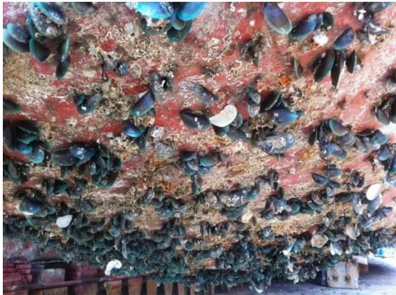
Image: Underside of a vessel hull, fouled with mussels, source Biofouling Solutions (A. Coutts)
