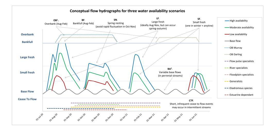
Figure 3. Conceptual flow hydrographs for three water availability scenarios (High, Moderate, and Low). Breeding season windows for each functional group of Southern MDB fishes are identified by dashed lines. Ecologically significant flow components which may promote key life history elements for fish (such as movement, spawning and condition) are labelled Bank full (BF), Overbank (OB), Large Fresh (LF), Spring nesting component (SN), Small Fresh (SF), Base flow (BA) and Cease-to-flow (CTF).
