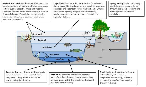
Figure 2. Ecologically significant components of the within-channel flow regime (including Cease to flow, Base Flows, Small Fresh, Large Fresh, Spring nesting component, Bank full and Overbank flows).
