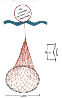
Mesh size cannot be less than 13mm measured on the diagonal.
