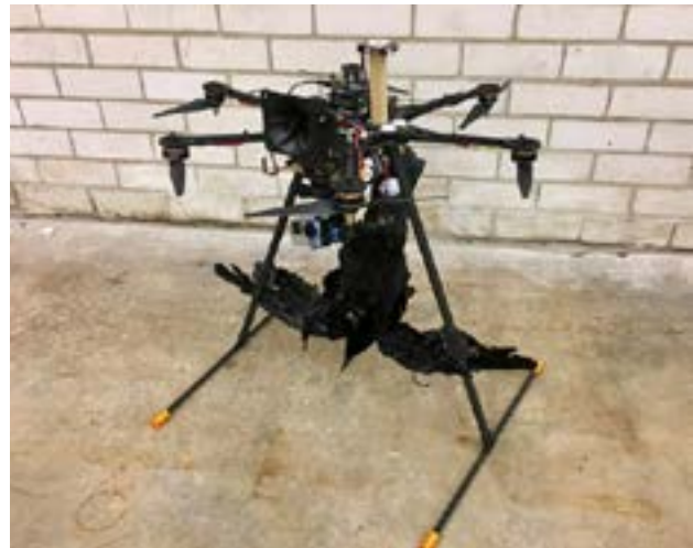
Figure 46. UAV equipped with horn tweeter and taxidermied crow.
