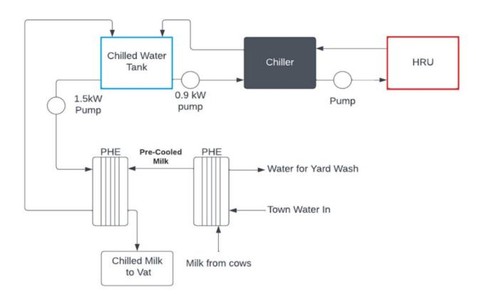
**MVD:** an extra PHE using glycol was installed to allow for future expansion; this system has higher "losses"
