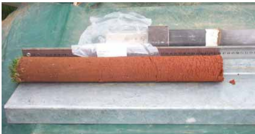
Figure 25. Intact soil core to be sectioned into 0-5, 5-10, 10-20, 20-30 and 30-40 cm increments.
