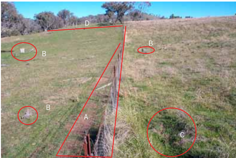
Figure 6. Soil sampling for soil organic carbon by avoiding “unrepresentative” areas, e.g. close to the fence (A), old tree stumps (B), visibly disturbed areas (C) and areas close to existing trees (D).
