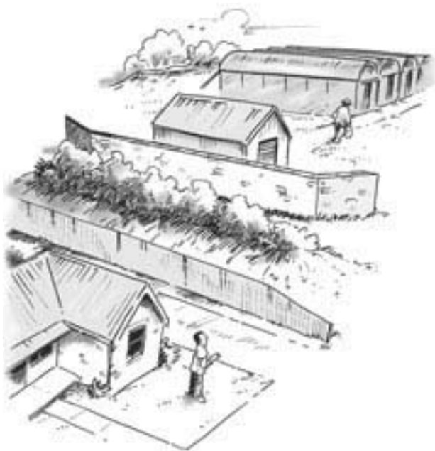
Noise barriers can be used to address potential problems with noisy equipment and machinery.
