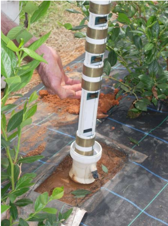
Figure 9. Enviroscan showing electronic sensors at various depths
