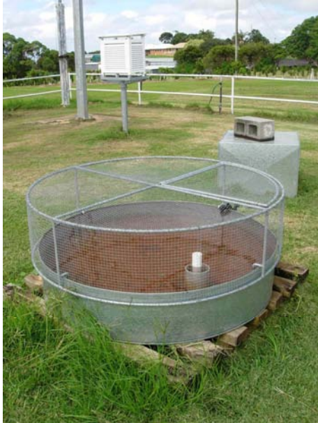
Figure 10. A class A pan measures evaporation
