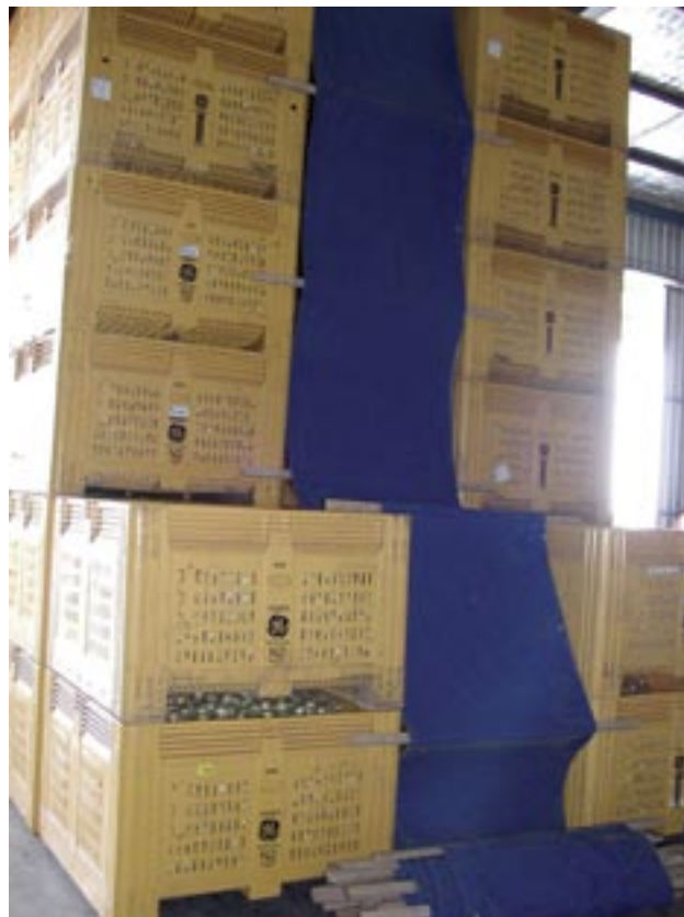
Forced air tunnel curing systems are a cost-effective method of removing field moisture and curing the outer skins of onions harvested in the Riverina summer.
