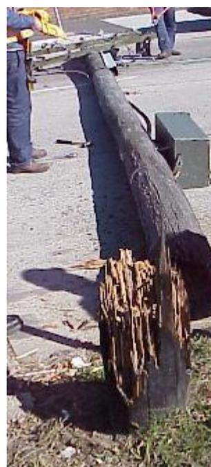
**Figure 1. Power pole failure resulting from termite attack.**
