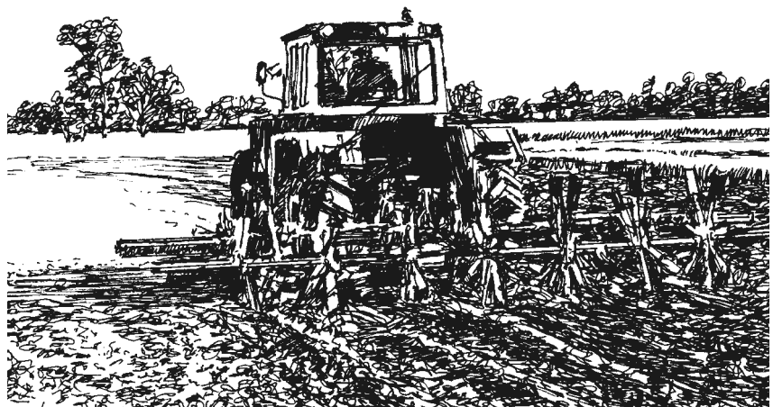
Figure D9-4. An implement for increasing surface roughness on a hardsetting soil
