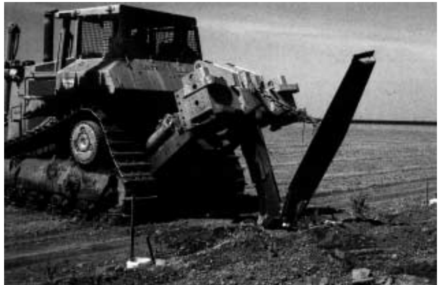
Figure D2-5. A Californian slip plough, which brings subsoil clay to the soil surface from a depth of about 1 m.
