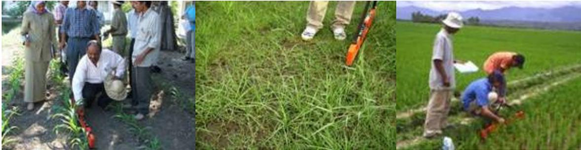
Figure 9: Random error is determined by using the EM38 in three different conditions; dry soil surface (left), saturated and flooded (right)
