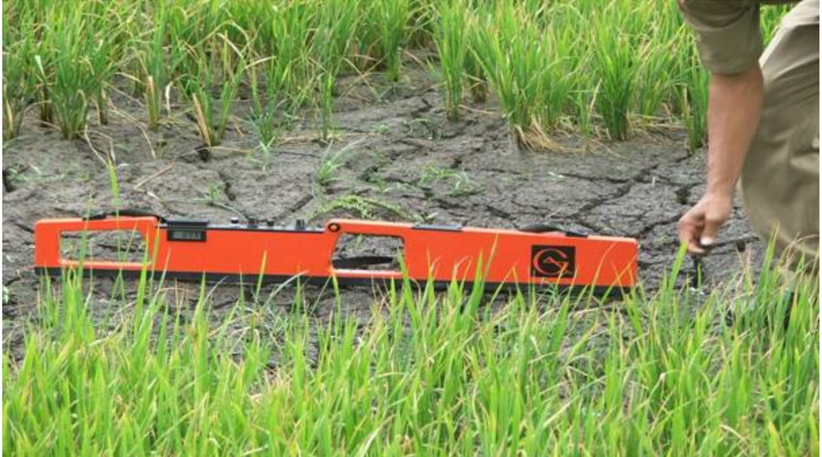
Figure 8: The EM38 being used in the field
