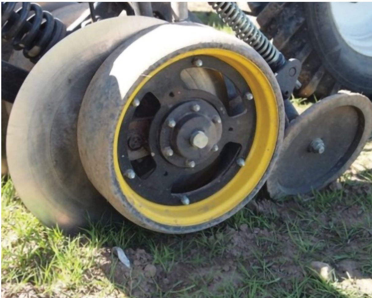
Figure 2. Disc seeders provide more uniform seed depth.
