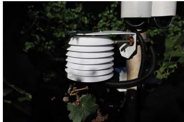
Figure 23. A temperature/humidity sensor.
