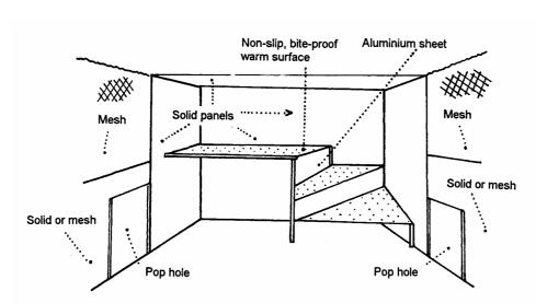
A design for laboratory dog housing incorporating a high platform accessible by steps (after Serpell, 1995).
