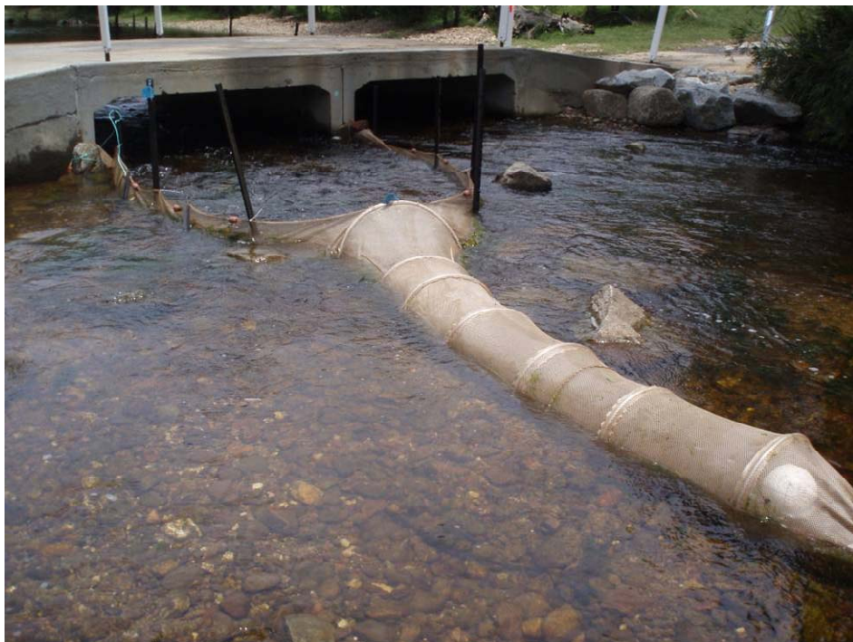
Figure 11. Fyke net configuration for trapping fish a) approaching, and b) exiting culvert.
