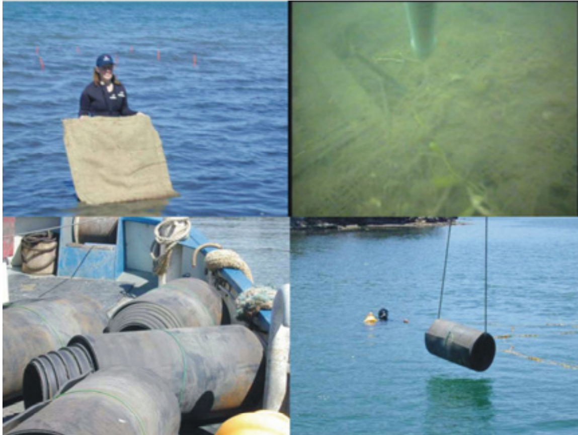
Plate 7. Trials in NSW to evaluate the feasibility of killing C. taxifolia by smothering it with various materials. Top left: jute matting about to be laid at Mannering Park in Lake Macquarie; top right: jute matting at Careel Bay after several months on the bottom; bottom left and right: rubber conveyor belting being laid in Lake Macquarie.
