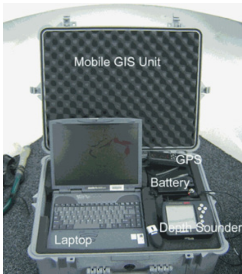
Plate 2. The on board mapping system developed to document the spatial extent of C. taxifolia infestations in NSW waterways.
