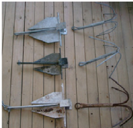
Plate 6. Sand and rock anchors used in experiments examining the effect of anchors. Two replicate lengths of chain and two replicate lengths of rope were attached, in separate trials, to each anchor.
