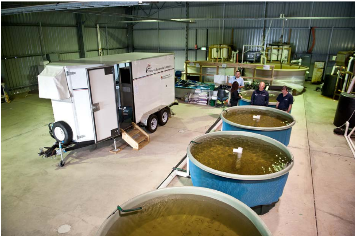
Figure 2. Experimental facilities at the Port Stephens Fisheries Institute showing 2000-L tanks in which juvenile fish were housed, adjacent to the mobile laboratory containing the hypo/hyperbaric chambers
