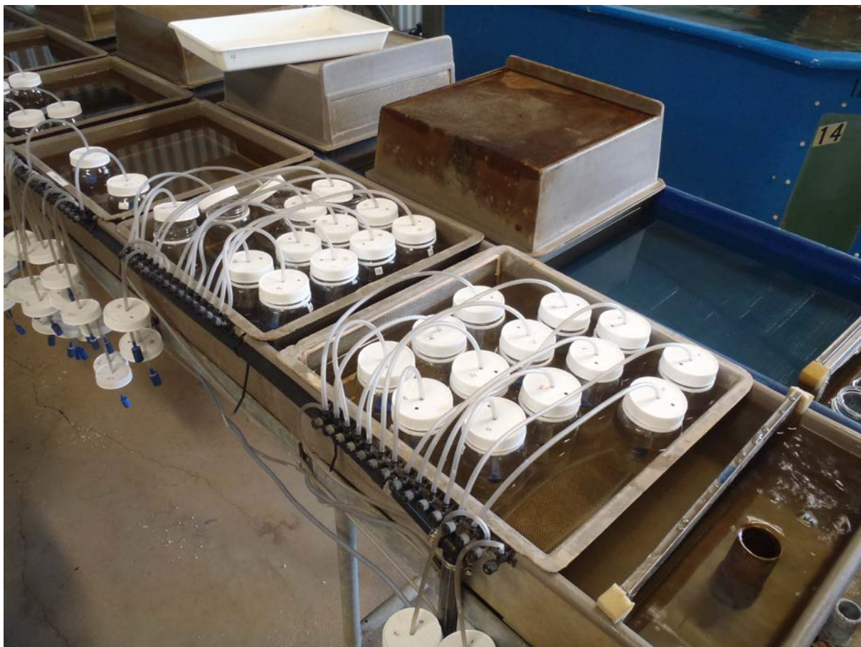
Figure 7. Aerated jars used to hold test groups of eggs and larvae before and after decompression in the chambers
