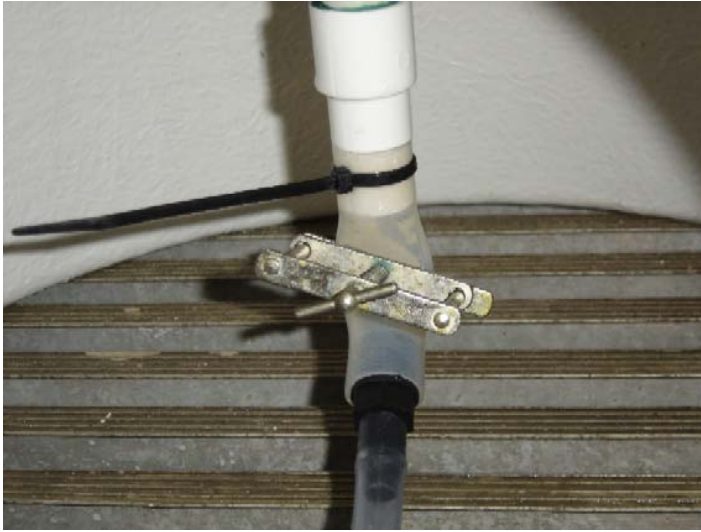
Fig 6. Outlet of the rearing vessel showing the air inlet controlled by a clamp that can also be used as a water outlet for draining the tank.
