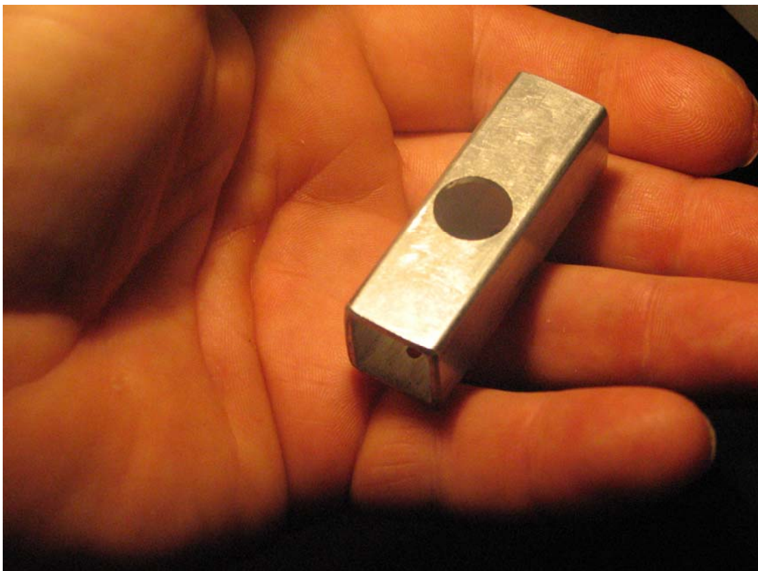
Figure 1. Individual 55 x 16 x 16 mm aluminium release capsule. Note 12 mm entrance portal and 1.5 mm drain holes.
