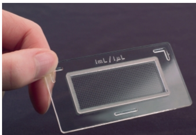
Fig 13. Sedgewick rafter style slide used for counting larvae.
