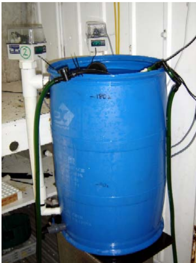
Fig 4. Water heating unit fashioned from a plastic drum with two thermostatically controlled heaters, a float valve and outflow tap (controlled by a pump).
