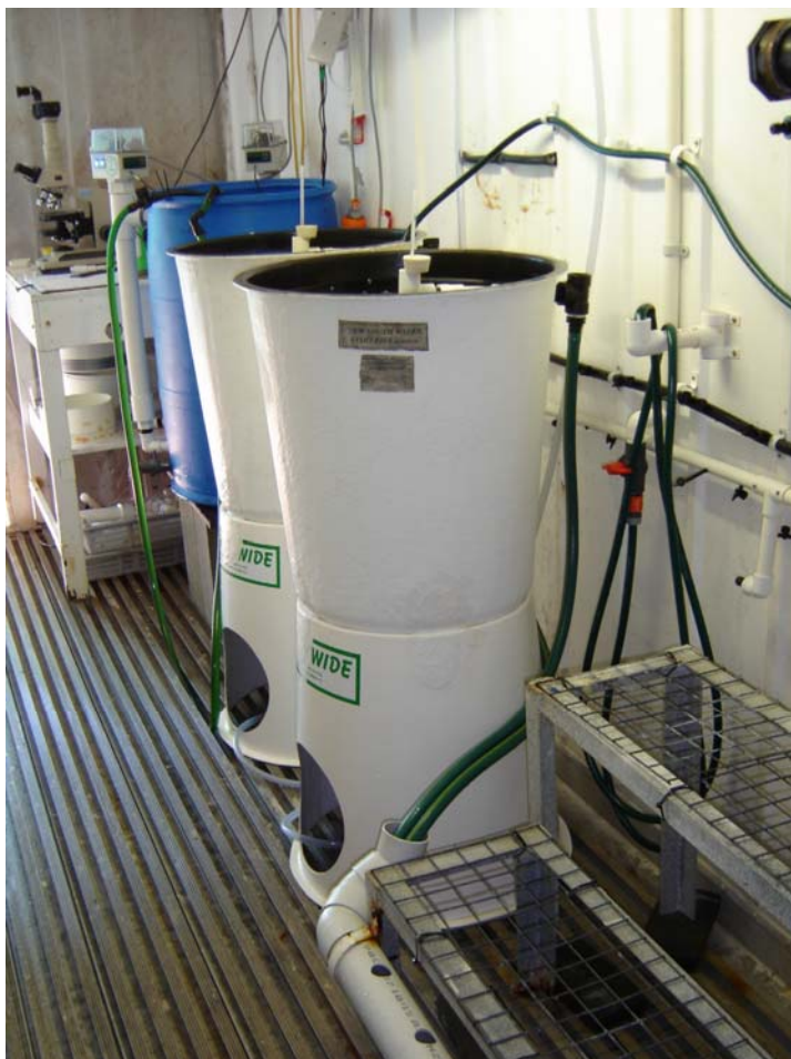
Fig 5. Two fibreglass larval rearing vessels on stands, showing overflow tube and top of the banjo screen (protruding from the banjo screens are thermometers).
