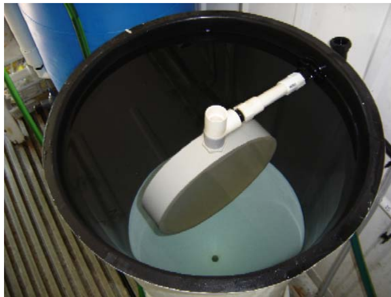
Fig 7. Banjo screen fitted to the over flow of a larval rearing vessel (note the conical bottom of the vessel).
