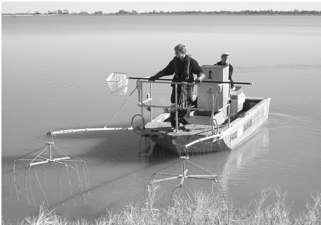
Figure 2.2. Staff undertaking boat electrofishing surveys to document the structure of fish communities in irrigation systems. (Photo: Charlotte Grove, NSW DPI).
