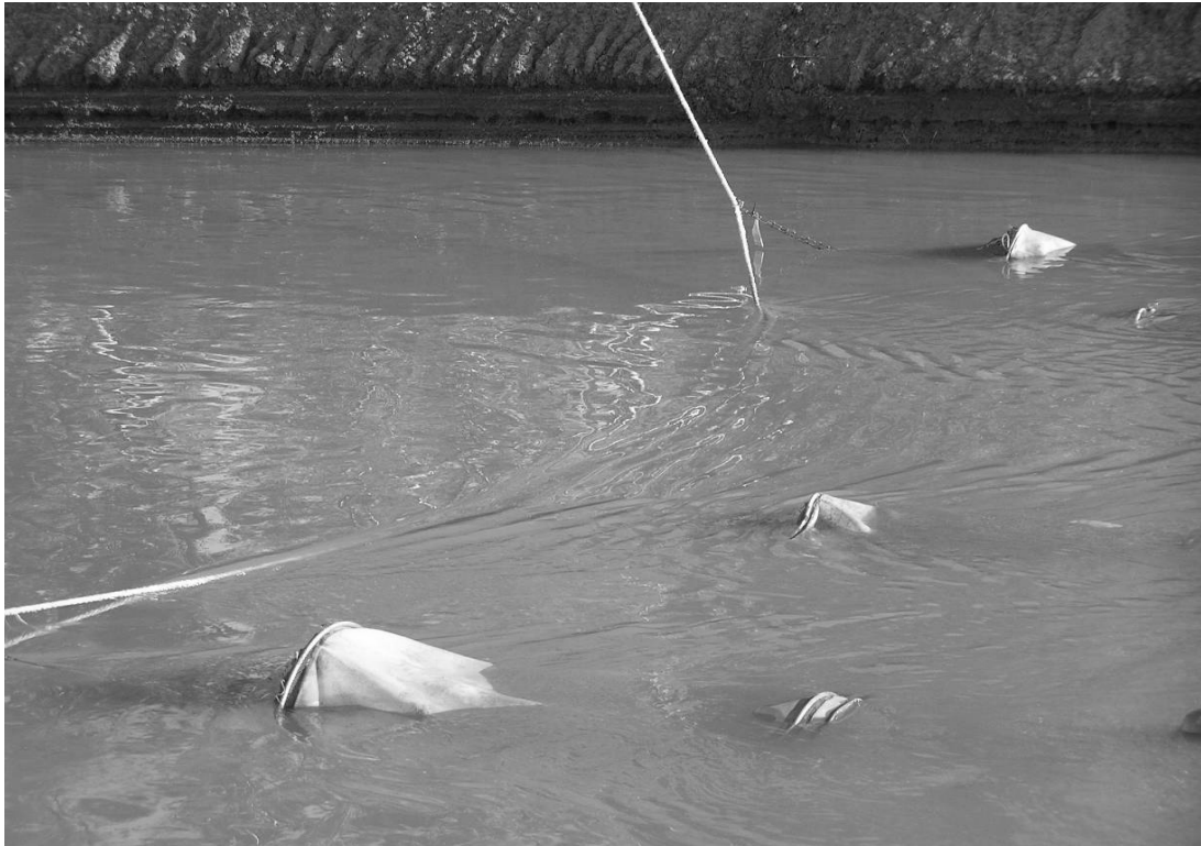
Figure 2.1. A typical deployment of larval sampling nets to collect drifting fish larvae in an irrigation canal. (Photo: Leo Cameron, NSW DPI).
