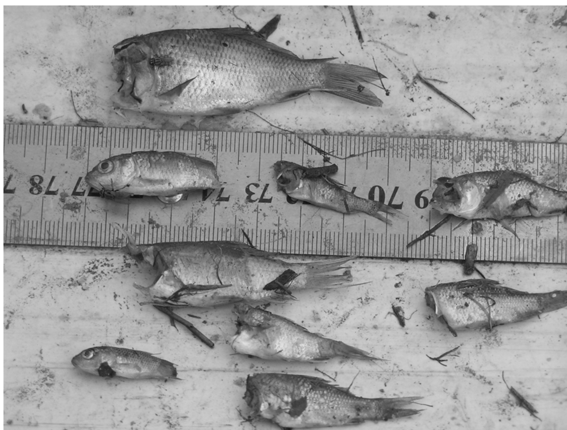
Figure 4.9. An example of fish injuries sustained during passage through a pump system on the Namoi River.
