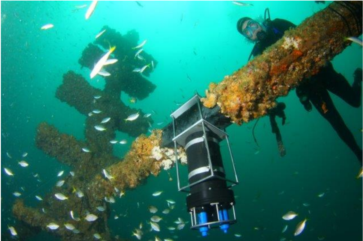
Figure 21. Vemco VR4 with a 10 year battery life and remote download capabilities fitted to the Sydney offshore artificial reef
