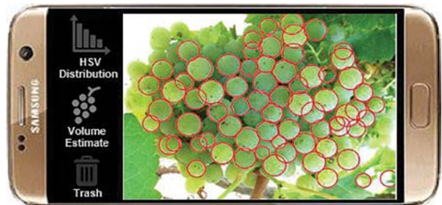
Figure 2: Prototype app running on android phone. After an image is taken in the vineyard, the app calculates berry volume and provides information on the number of berries per size category.
