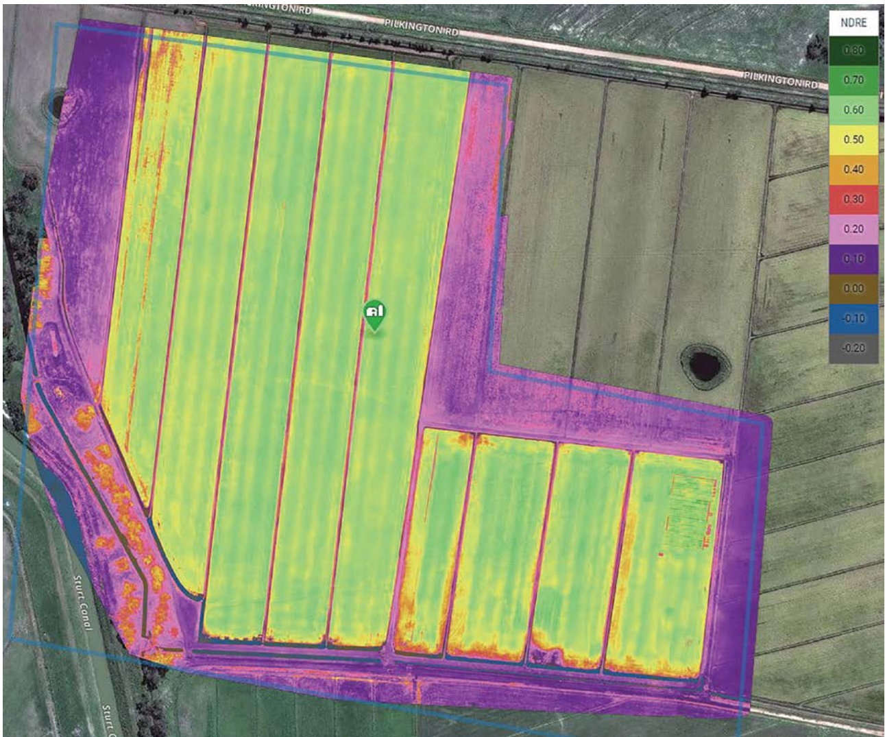
Figure 2. High-resolution multispectral drone data, in this case NDRE, shows the impact of non-uniform top-dress spreading. The non-uniform spreading pattern can be seen running up and down the bays. IMAGE: John Hornbuckle
