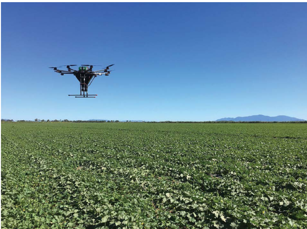
Figure 4. AeroBugs drone delivering beneficials to a melon crop (photo by Dan Papacek)
