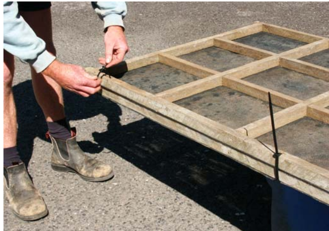
Figure 4. Spat bearing tray and lid tray being tied together through aligned holes drilled in the tray frames.
