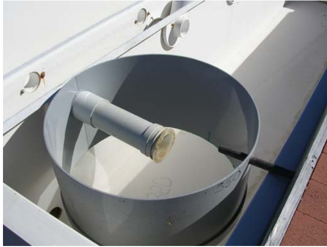
Figure 2. 45 cm diameter upweller screen fitted with 0.35 mm mesh, with an outlet screen and a support peg.
