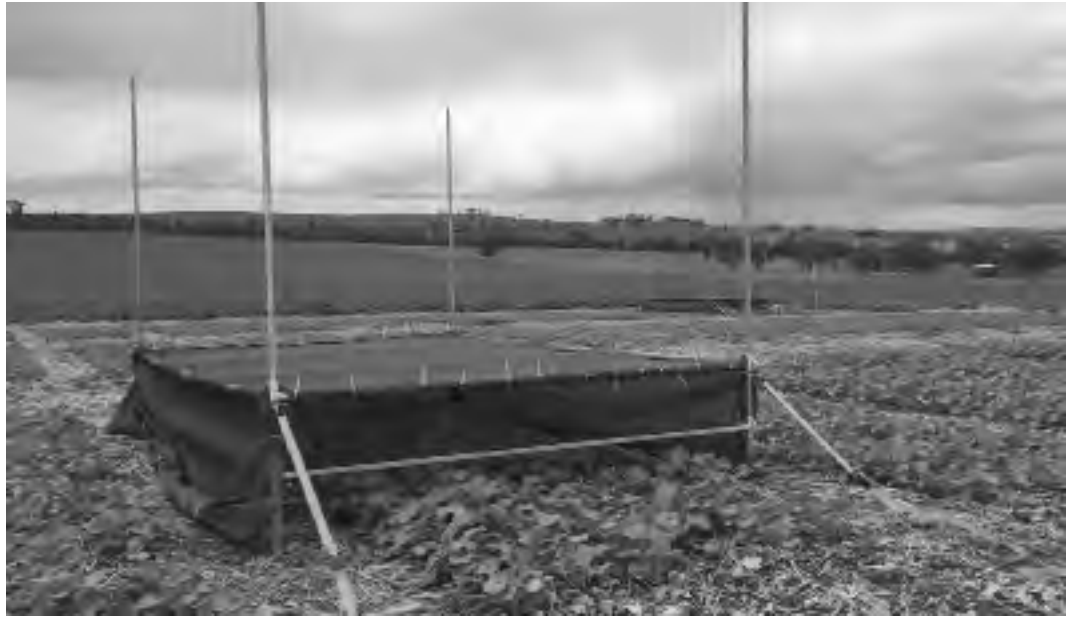
Figure 2. Shade shelter on canola critical growth period experiment at Wagga Wagga on 23 June 2016. The lid was made to slide up the four corner poles throughout the year and remain approximately 50 cm above the crop canopy.
