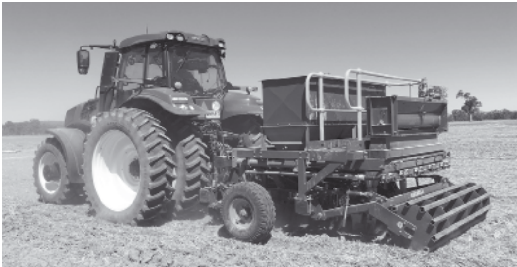
Figure 2. 3-D Ripping Machine, designed and fabricated by NSW Department of Primary Industries staff. (Photo by Guangdi Li)
