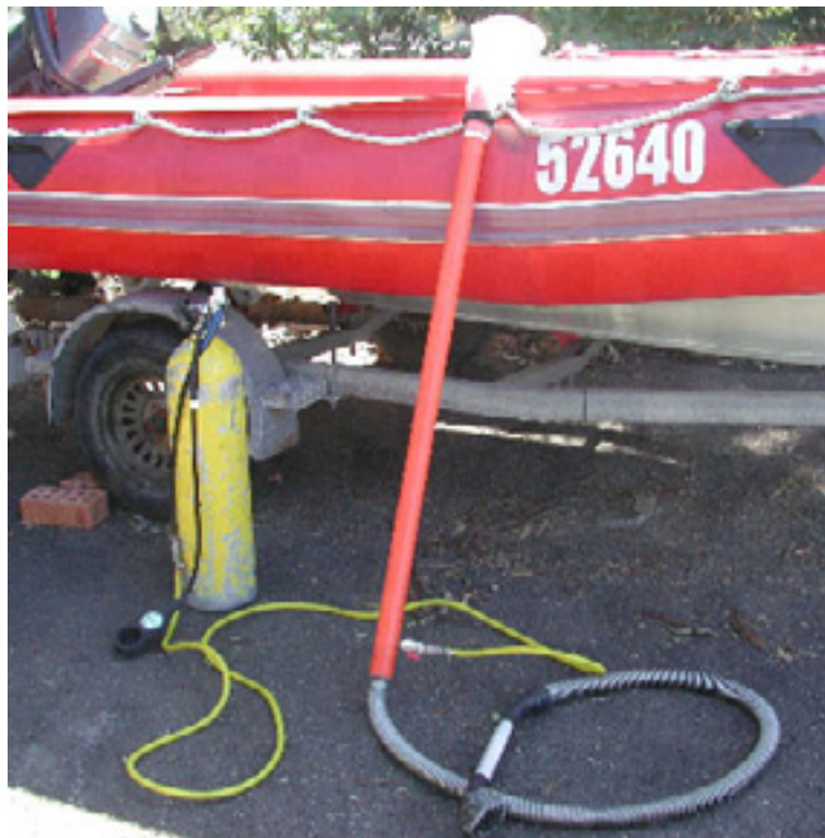
Plate 1. The venturi sampler consisting of a 1500 mm length of 40 mm diameter PVC tube (orange tube), high pressure hose fitting with ball valve switch near the lower end of the tube, length of 45 mm diameter, flexible hose (grey hose) with brush attachment and at the opposite end of the orange tube, the mesh (180 \mu m) sample bag with velcro strap.
