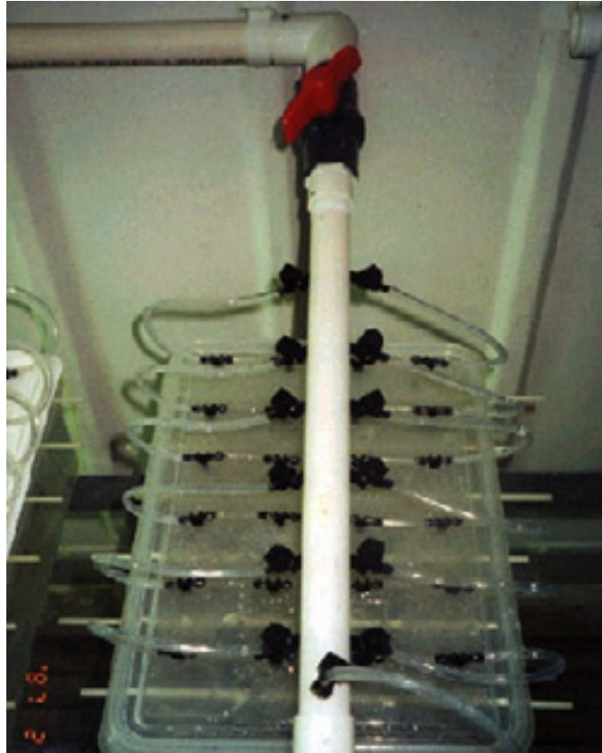
Plate 1. One module of the miniature down-welling system showing 6 rows of down-welling units each with its own supply of water.
