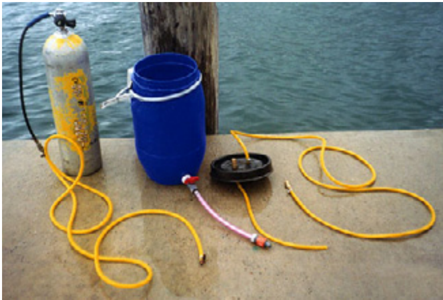
Plate 1. The deployment pump consisting of a 35 L drum with hose, the lid with in coming (short hose, without air stone attached) and out going (hose connected and fitted with pressure relief valve) couplings and SCUBA tank with high pressure (in coming) hose.
